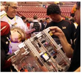
of a typical hardware inspection items include: the size of the robot, safety standards for the hardware (e.g. no sharp edges or corners), and ensuring the robot contains official build components. The Robot Inspector will also check the robot controller to confirm that it is named appropriately, has the correct Android Operating System installed, and that robot controller app is the default application being used to connect to the core robot modules.
